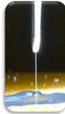
This aerosol-based approach is flexible in its ability to support a wide viscosity range of inks, produce both thin & thick layers, and print both small & large features. Its non-contact process can tolerate a variable stand-off distance (1-5mm) and variable angle of incidence (up to  $\pm 22.5$  degrees from normal) making the process readily suited for printing on non-planar and 3-dimensional substrates.
